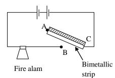
c) The bimetallic strip indicated by AC in the above figure is made by riveting a strip of iron and a strip of brass together.
