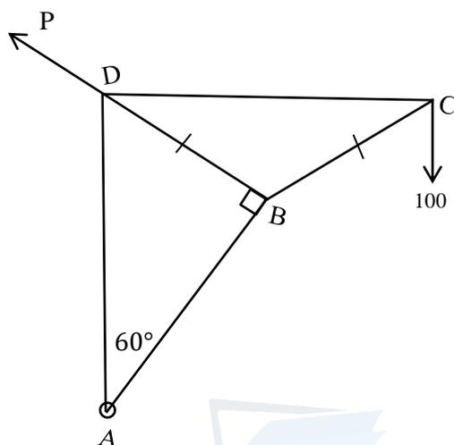
The figure shows a framework made by joining light rods AB, BC, CD, BD and AD. It is smoothly hinged at A and kept at equilibrium such that AD is vertical and DC is horizontal, by applying a force  $P$  along  $\overrightarrow{BD}$  and hanging a weight of 100 N at C
