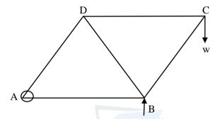
The frame work shown in the diagram is made by AB, BC, CD, DA and DB of light equal rods, hinged at A, supported at B and and a weight w is hung from C, AB is horizontal.
