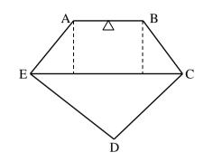
The uniform rods of weight W such that AB = AE = BC = 2a, CD = DE = 4a. These are joined smoothly as shown in the figure and is kept in equilibrium by a wedge in the midpoint of AB and a light rod of length joined to the point C, E.
