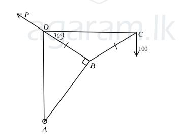
The frame work made up of light rods is hinged at the joint A as shown in the figure. A force P act on D in the direction BD and a weight of 100 N is hanged at C So that DC is horizontal and AD is vertical.
